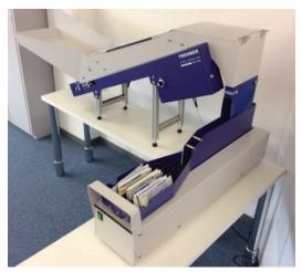
Banknote bundling machine is used for processing unstacked cash coming in bags used for deposit machines (ADM) and for merchant cash collection.
